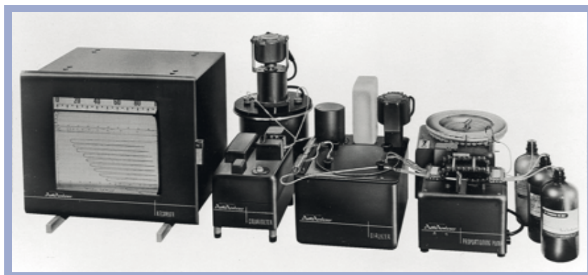
Figure 1. The Technician AutoAnalyzer 1. From right to left: reagents, autosampler (rear), peristaltic pump (fluidics), dialyser (protein removal), incubator (rear), double-beam spectrophotometer (front), chart record. Images courtesy of manufacturers.
