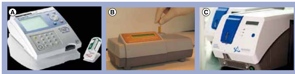
Figure 14. Point-of-care immunoassay platforms. (A) Alere Triage system. (B) LifeAssays system. (C) Avantra Q400 Multiplex biomarker system. Images courtesy of manufacturers.
